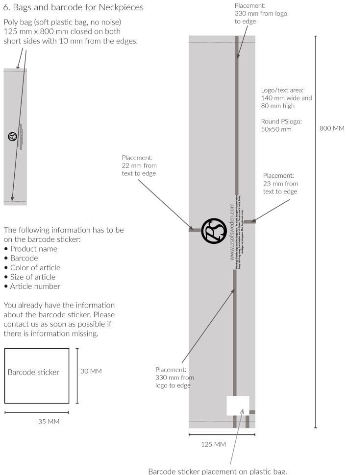
Barcode sticker placement on plastic bag. 20 mm from bottom and 10 mm from the left hand side, on the right hand side of the bag. Size of the barcode sticker is 30 mm wide x 35 mm long.
