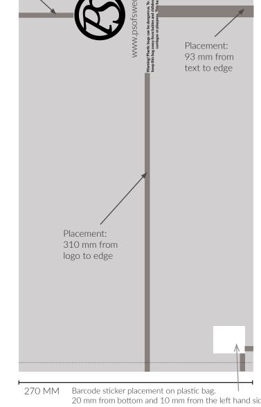
Barcode sticker placement on plastic bag. 20 mm from bottom and 10 mm from the left hand side, on the right hand side of the bag. Size of the barcode sticker is 30 mm wide x 35 mm long.
