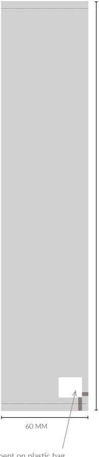
Barcode sticker placement on plastic bag. 20 mm from bottom and 10 mm from the left hand side, on the right hand side of the bag. Size of the barcode sticker is 30 mm wide x 35 mm long.
